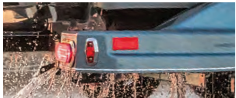
Submersible, angled LED backup lights for long life & improved visibility
