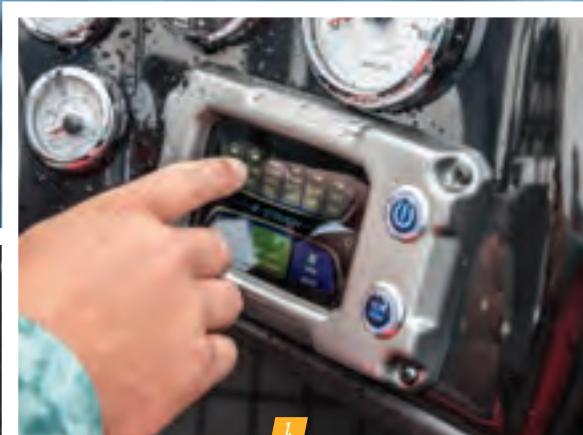
1. NEW touchscreen switch panel w/1-touch boat controls including First Fish, Nite Mode, master power, trim, lighting, bilge, livewells & more 2. 3-level center rod locker for rods up to 8' (2.44 m) w/tapered rod tubes to protect rod tips 3. Aft 26-gal. (98.42 L) GUARDIAN™, anti-slosh livewell & bow 5.5-gal. (20.82 L) baitwell w/bucket
