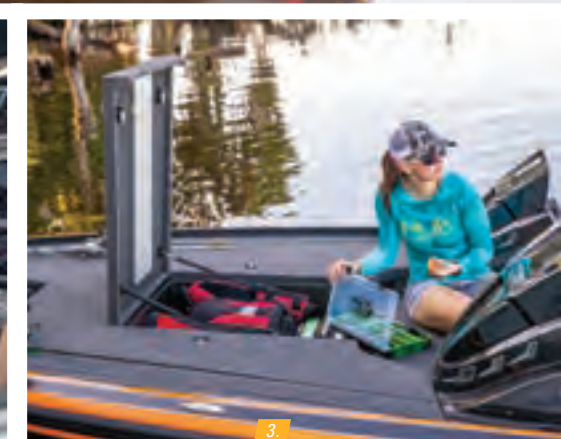
1. Z-CORE™ seating system w/Force Flex suspension & contoured, rotomolded frame for driver & passenger 2. Step to bow deck w/62-qt. (58.67 L) insulated cooler & removable trash receptacle 3. Oversized lockable bow center storage locker w/piston-lift assist
