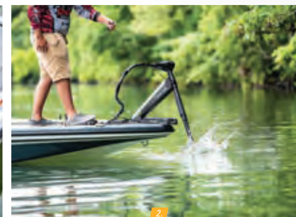
1. Driver & passenger bucket seats w/molded-in, gelcoated storage below each 2. Minn Kota® Edge® 12V, 55-lb. (24.95 kg) thrust, 45" (1.14 m) shaft foot-control trolling motor 3. Custom-molded modular console w/2-tone gelcoat w/Lowrance® HOOK² 4x fishfinder
